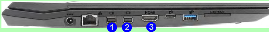
Figure 1 - 18 - Left Side View (Mini Display Ports & HDMI Port Highlighted) - Single Model Pictured
